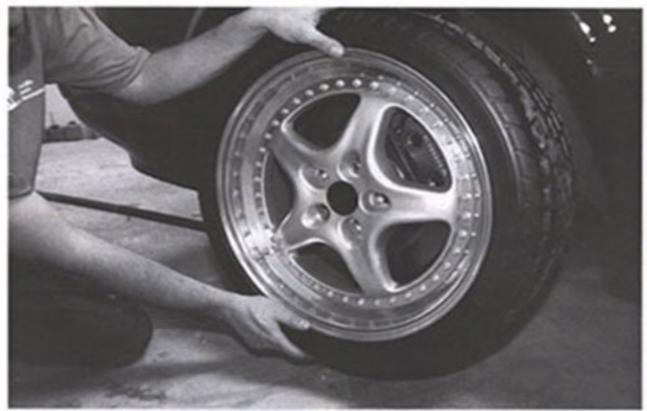
After one final spin, with the caliper pulled outboard as far as possible, we achieve clearance!
