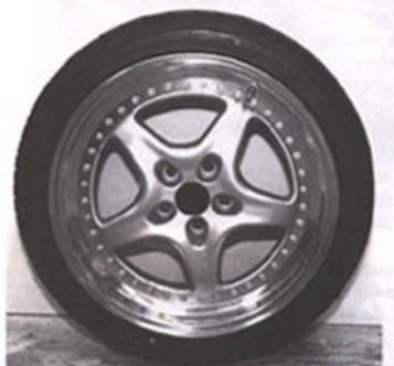
The attractive Speedline SL978 threepiece wheels were delivered with Dunlop SP 8000s, the same tires used by Saleen to achieve the high cornering forces generated by his race-winning 'Stangs.
