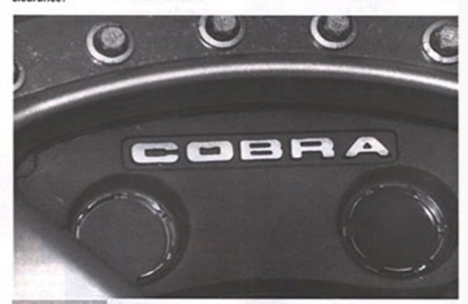
Note the tight fit, which actually looks really cool. We ended up with .13 inches of clearance, which is plenty: further driving and some high-speed cornering abuse and braking has not caused any problems.
