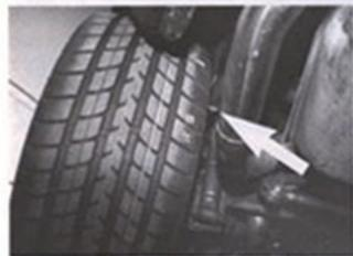
Checking for the typical interference points out back—the tailpipes and quad shocks (arrows)—we see that we have plenty of room for side-to-side movement of the rear axle. In cars not equipped with a panhard bar or Watt's linkage to eliminate such movement, it's best to leave about 1 inch between the wheel/tire and these two points to prevent damage and equipment failure.
